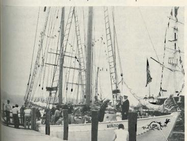
Rear Admiral Donald B. MacMillan stands on the bow of the schooner Bowdoin at her berth in Mystic Seaport. During the four years he was marooned in a North Greenland ice field, Admiral MacMillan conceived of a ship designed specifically for Arctic work. Built in 1920-21 and named for the Admiral's college, the Bowdoin, only 88 feet long and 21 feet wide, can be iammed into a niche among rocks when ice threatens.
